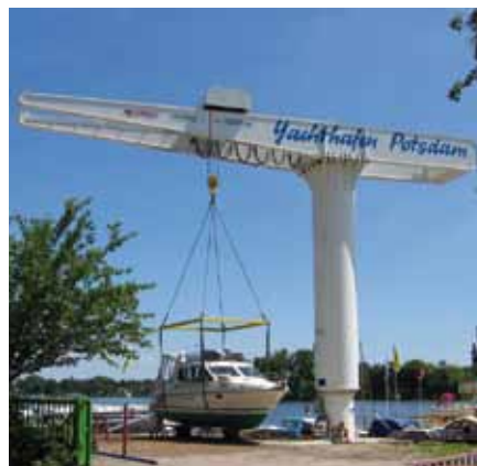
Type: BOSS / ZW Capacity: 25,000 / 6,300 kg Outreach: 6,500 / 12,500 mm Location: D-Potsdam / Havel
