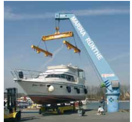
Type: MAAT Capacity: 16,000 kg Outreach: 6,000 mm Location: D-Bergkamen / Datteln-Hamm Kanal
