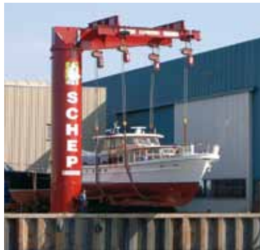
Type: BOSS Capacity: 4 x 10,000 kg Outreach: 6,250 mm Location: NL-Nieuwerkerk / IJssel
