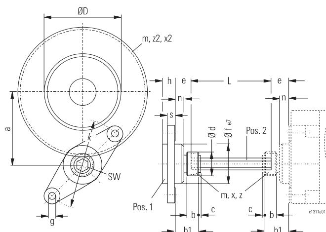
**Flange bearing with hexagonal shaft**
